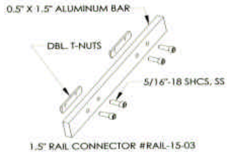
1.5" RAIL CONNECTOR #RAIL-15-03
